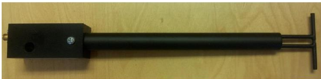
Figure 1 – MVG COMOSAR Validation Dipole
