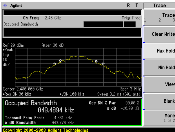
20dB Bandwidth plot on channel 78 (1Mbps)
