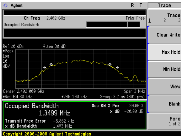
20dB Bandwidth plot on channel 39 (3Mbps)
