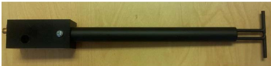
Figure 1 – MVG COMOSAR Validation Dipole
