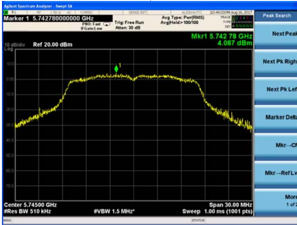
(802.11a) PSD plot on channel 157
