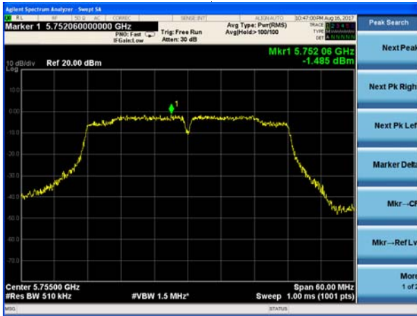
(802.11n40) PSD plot on channel 159
