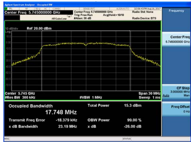
(802.11 AC20) -26dB&99%Bandwidth plot on channel 40
