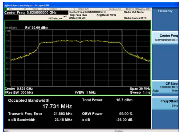
(802.11 AC20) -26dB&99%Bandwidth plot on channel 48
