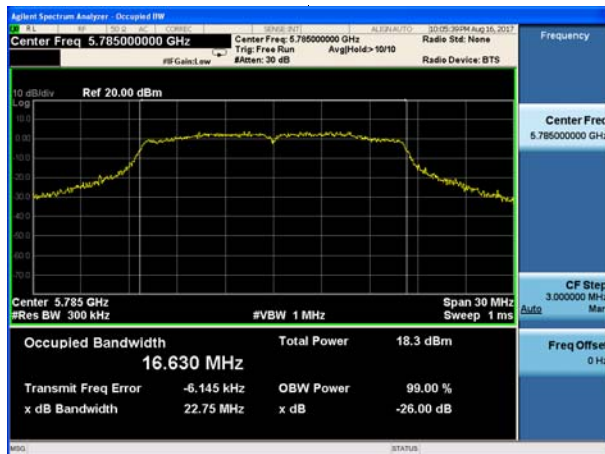
(802.11a) -26dB&99%Bandwidth plot on channel 48
