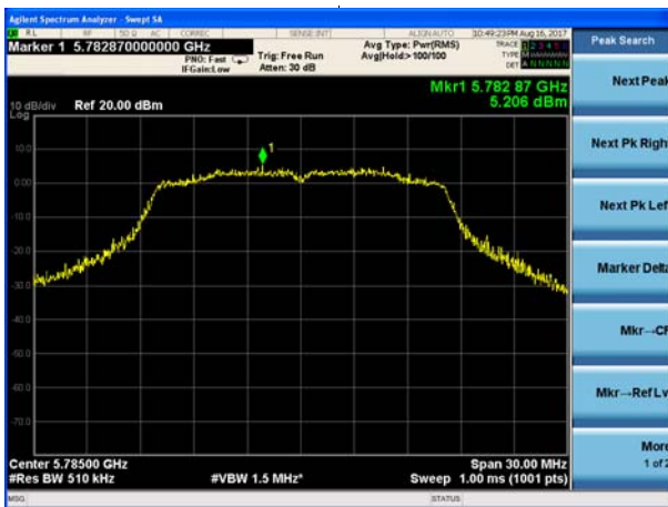
(802.11a) PSD plot on channel 165
