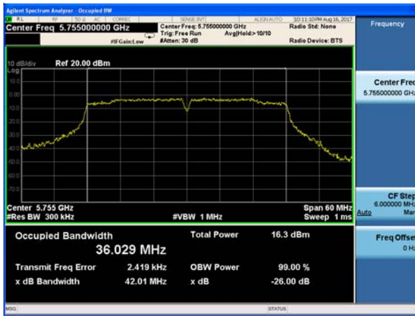
(802.11 n40) -26dB&99%Bandwidth plot on channel 46
