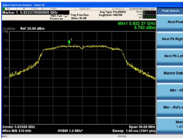
(802.11a) PSD plot on channel 165
