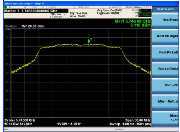
(802.11n20) PSD plot on channel 157
