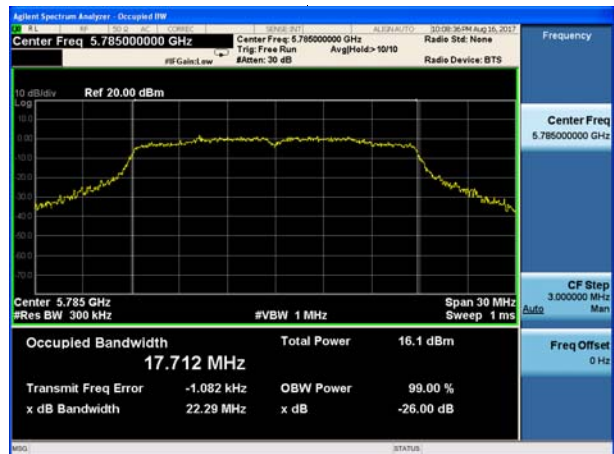
(802.11 n20) -26dB&99%Bandwidth plot on channel 48
