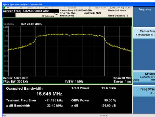
(802.11a) -26dB&99%Bandwidth plot on channel 48
