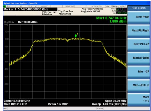
(802.11ac20) PSD plot on channel 157
