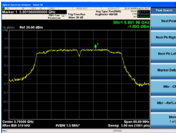
(802.11n40) PSD plot on channel 159
