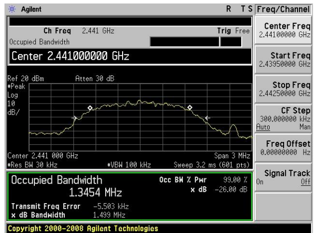
20dB Bandwidth plot on channel 39 (2Mbps)
