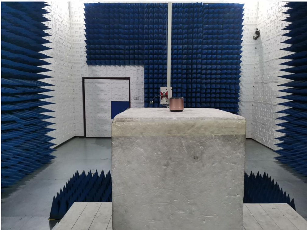
RADIATED EMISSION TEST SETUP ABOVE 1GHZ
