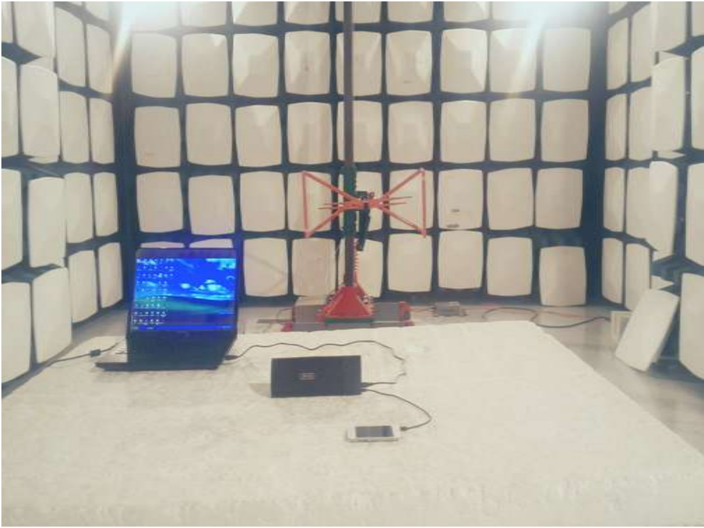
FCC RADIATED EMISSION TEST SETUP
