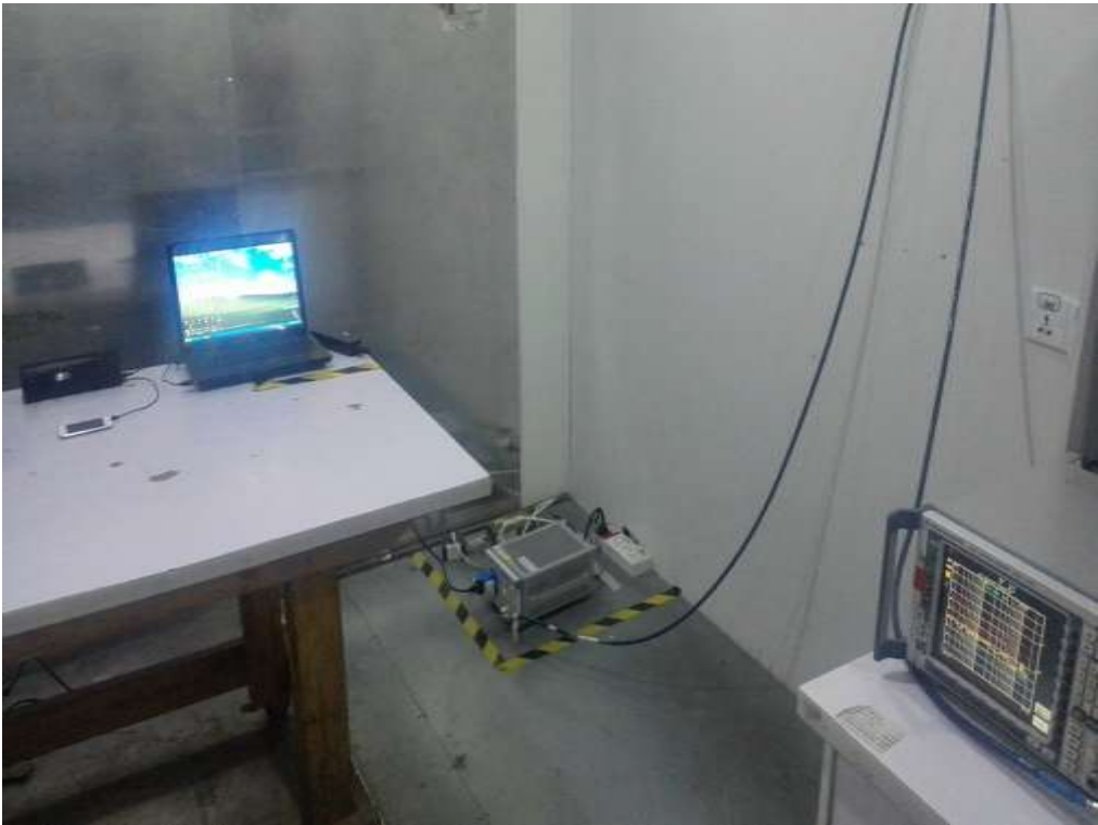
FCC RADIATED EMISSION TEST SETUP
