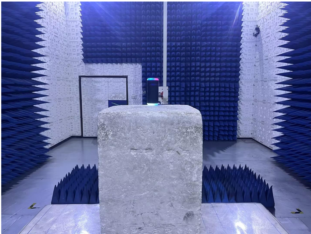
RADIATED EMISSION TEST SETUP ABOVE 1GHz
