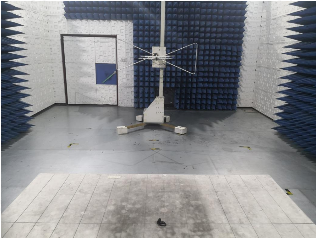
RADIATED EMISSION TEST SETUP ABOVE 1GHZ
