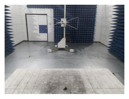
RADIATED EMISSION TEST SETUP ABOVE 1GHZ
