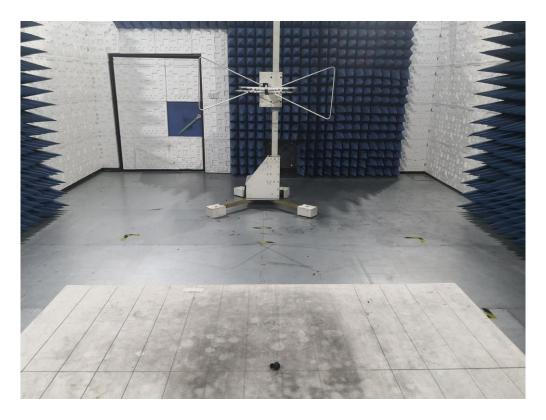
RADIATED EMISSION TEST SETUP ABOVE 1GHZ
