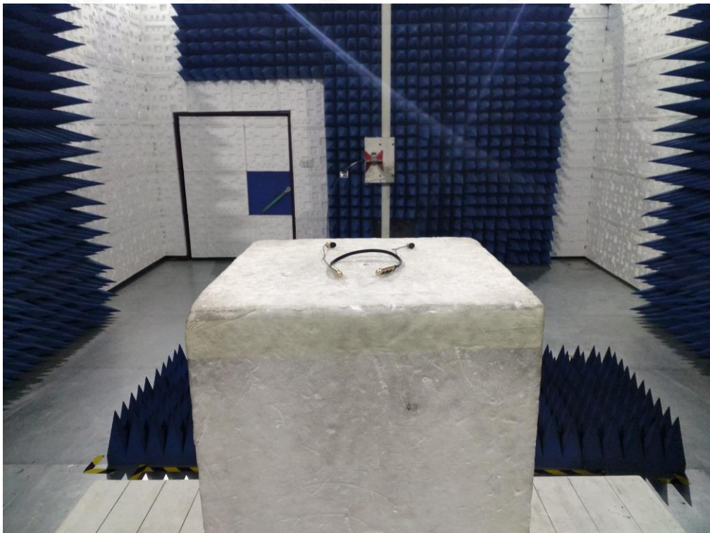
RADIATED EMISSION TEST SETUP ABOVE 1GHZ
