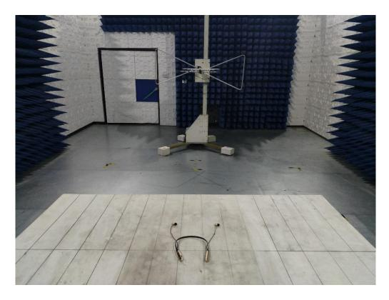
RADIATED EMISSION TEST SETUP ABOVE 1GHZ
