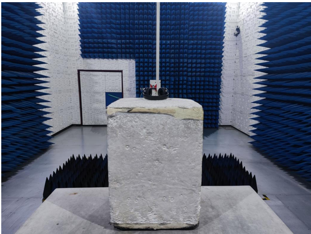
RADIATED EMISSION TEST SETUP ABOVE 1GHZ
