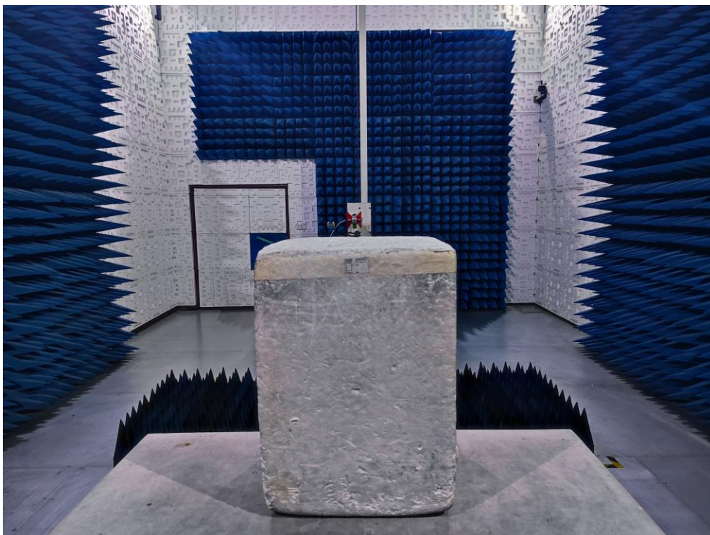
RADIATED EMISSION TEST SETUP ABOVE 1GHZ
