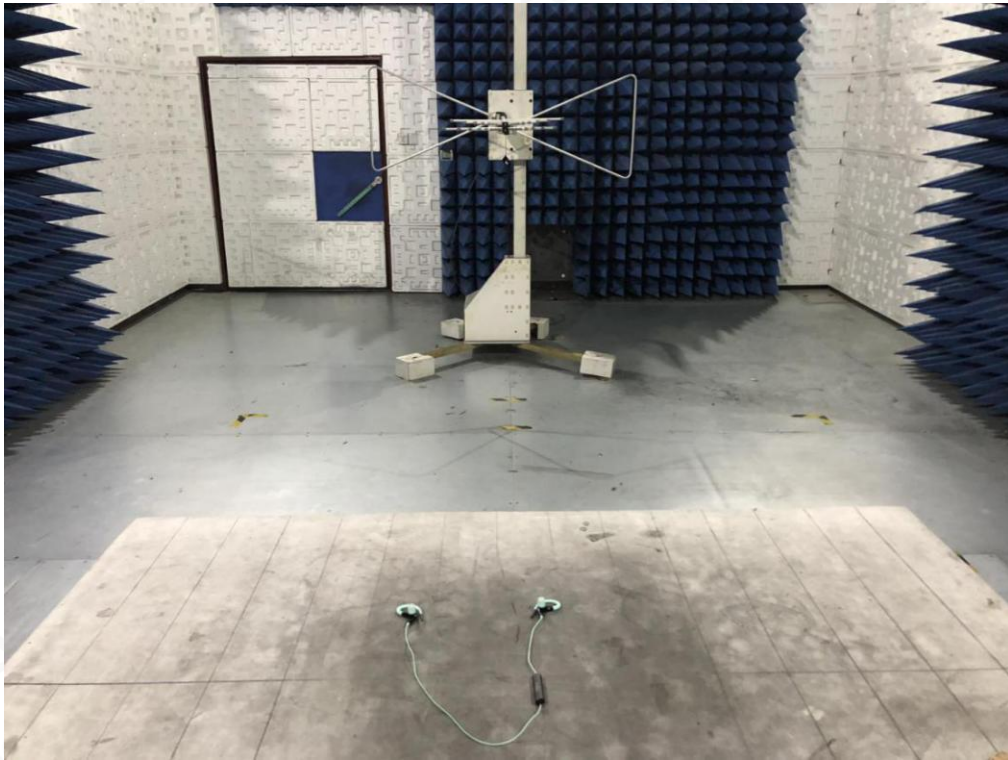
RADIATED EMISSION TEST SETUP ABOVE 1GHZ
