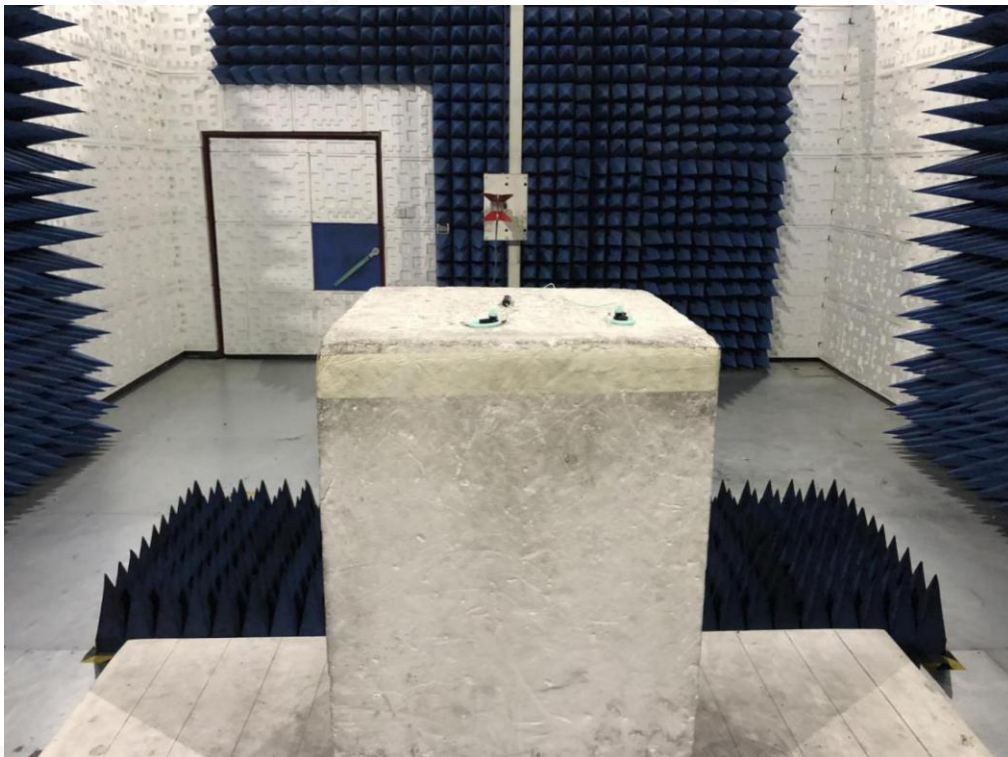
RADIATED EMISSION TEST SETUP ABOVE 1GHZ
