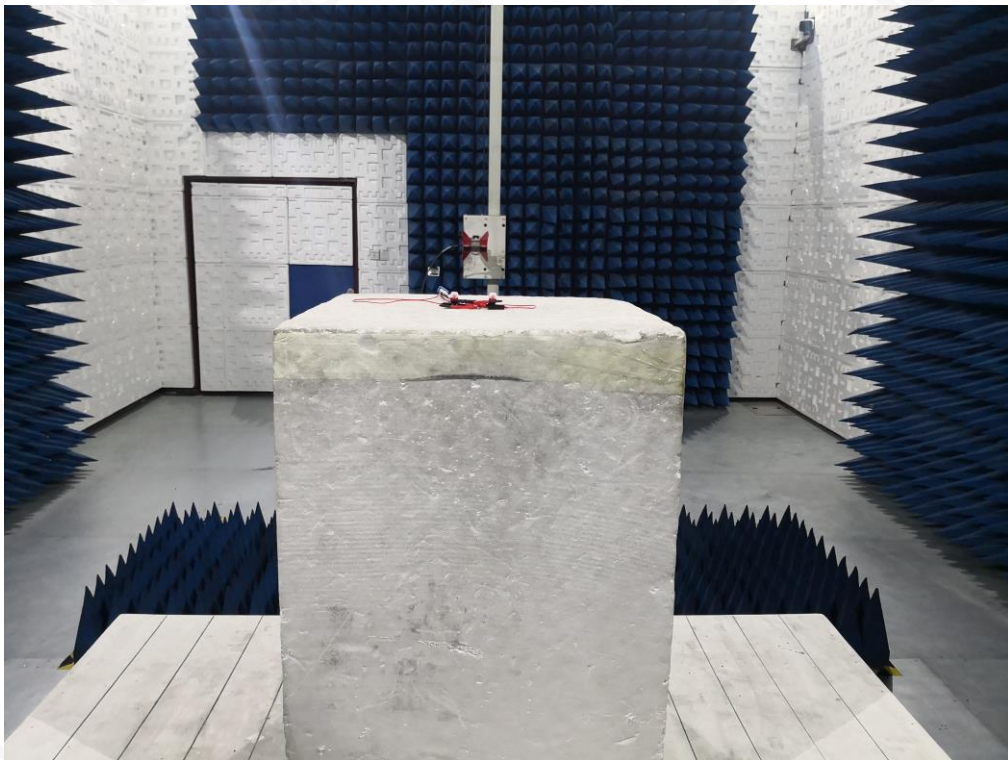
RADIATED EMISSION TEST SETUP ABOVE 1GHZ
