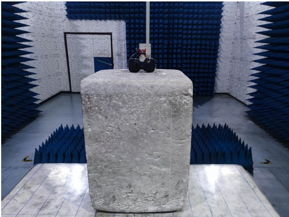
RADIATED EMISSION TEST SETUP ABOVE 1GHz
