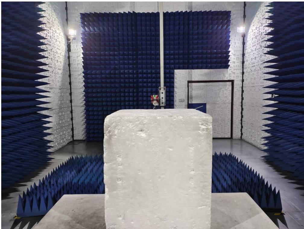
RADIATED EMISSION TEST SETUP ABOVE 1GHz
