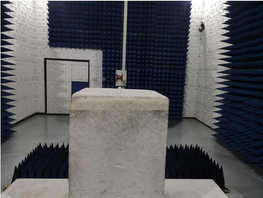
RADIATED EMISSION TEST SETUP ABOVE 1GHz
