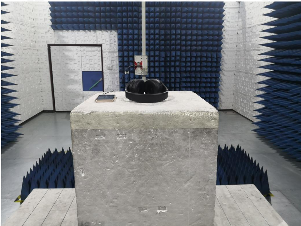
RADIATED EMISSION TEST SETUP ABOVE 1GHZ
