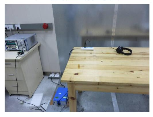
FCC RADIATED EMISSION TEST SETUP
