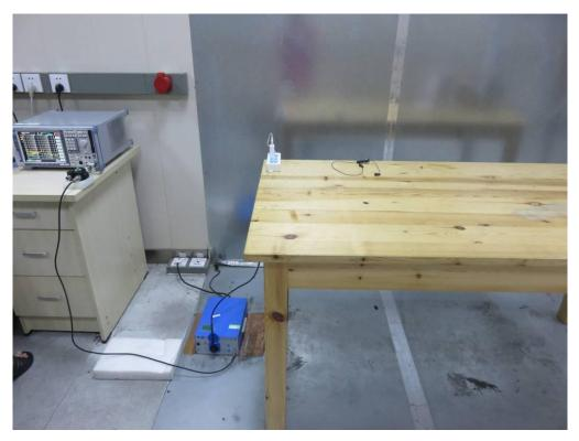
FCC RADIATED EMISSION TEST SETUP
