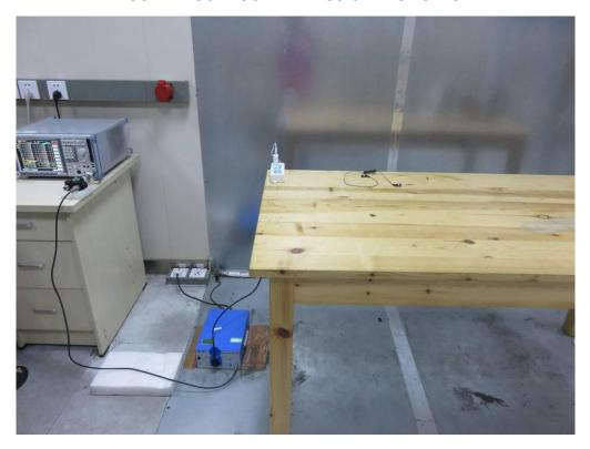
FCC RADIATED EMISSION TEST SETUP
