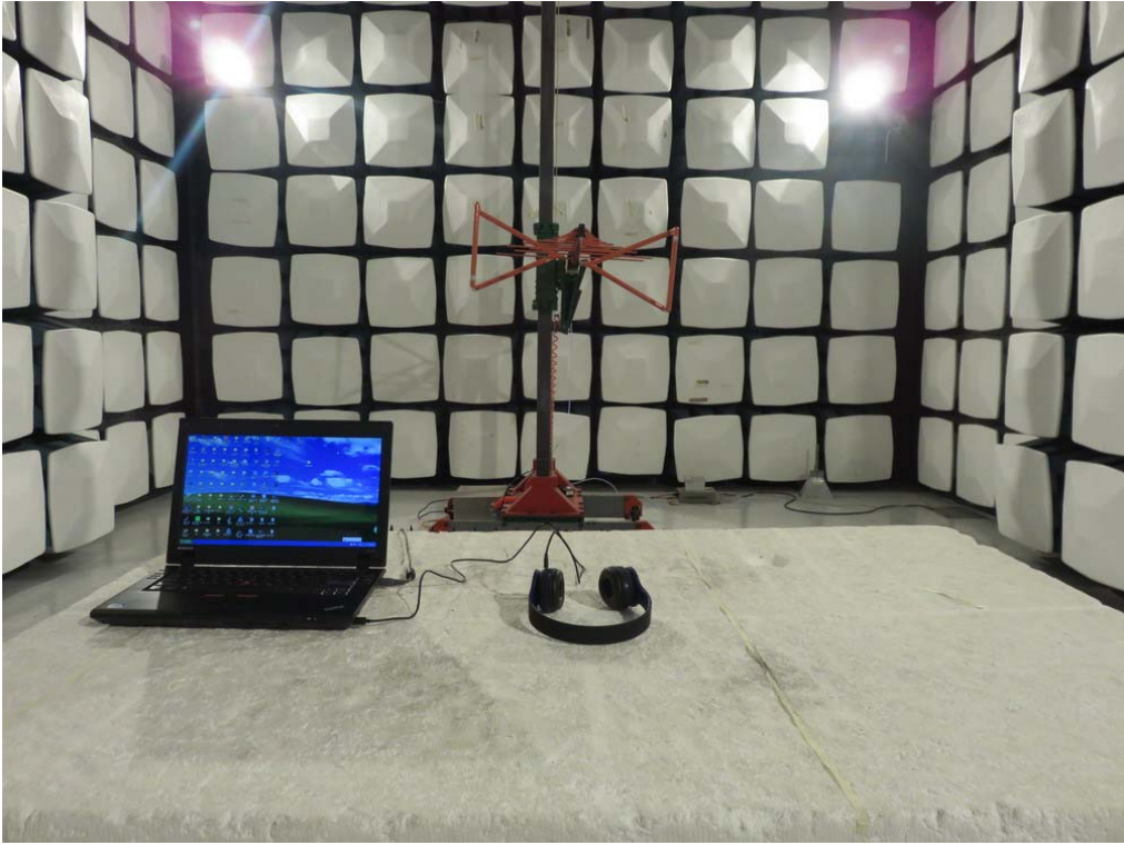
FCC RADIATED EMISSION TEST SETUP
