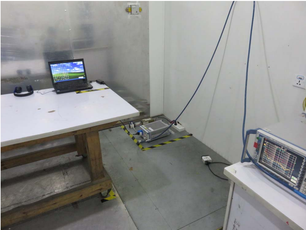
FCC RADIATED EMISSION TEST SETUP
