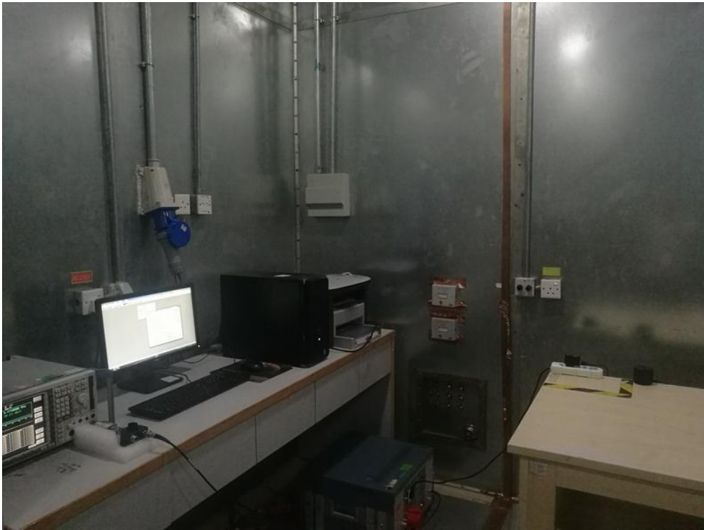
FCC RADIATED EMISSION TEST SETUP
