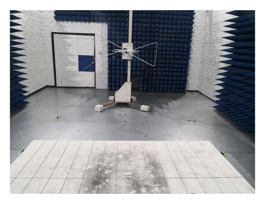
RADIATED EMISSION TEST SETUP ABOVE 1GHZ
