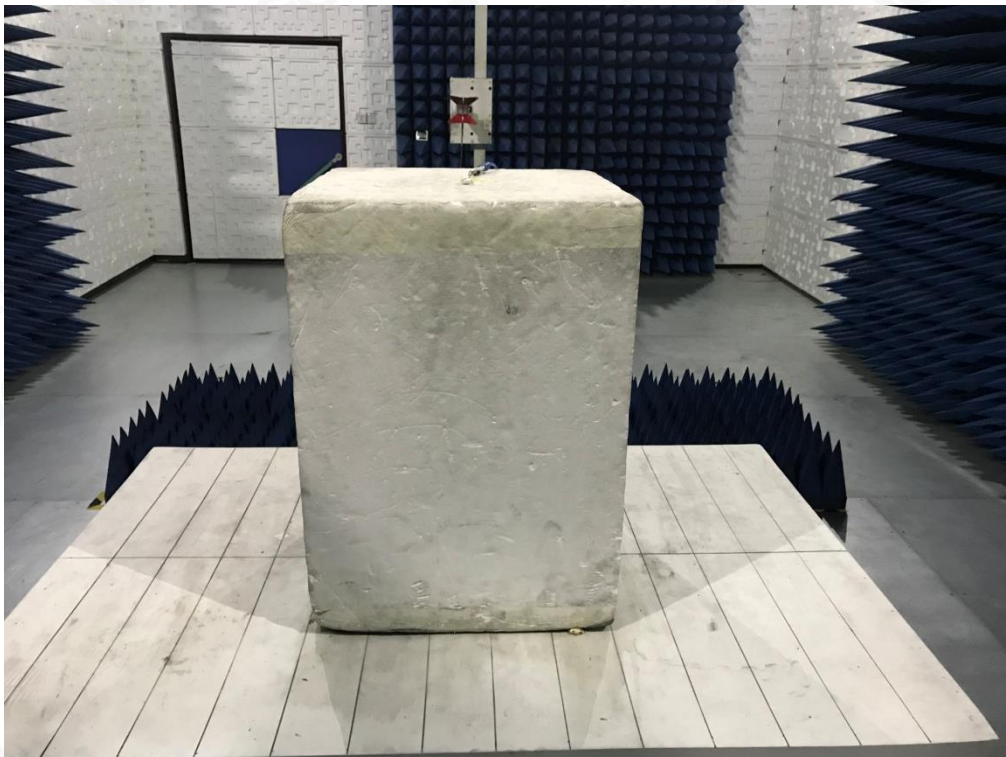
RADIATED EMISSION TEST SETUP ABOVE 1GHZ
