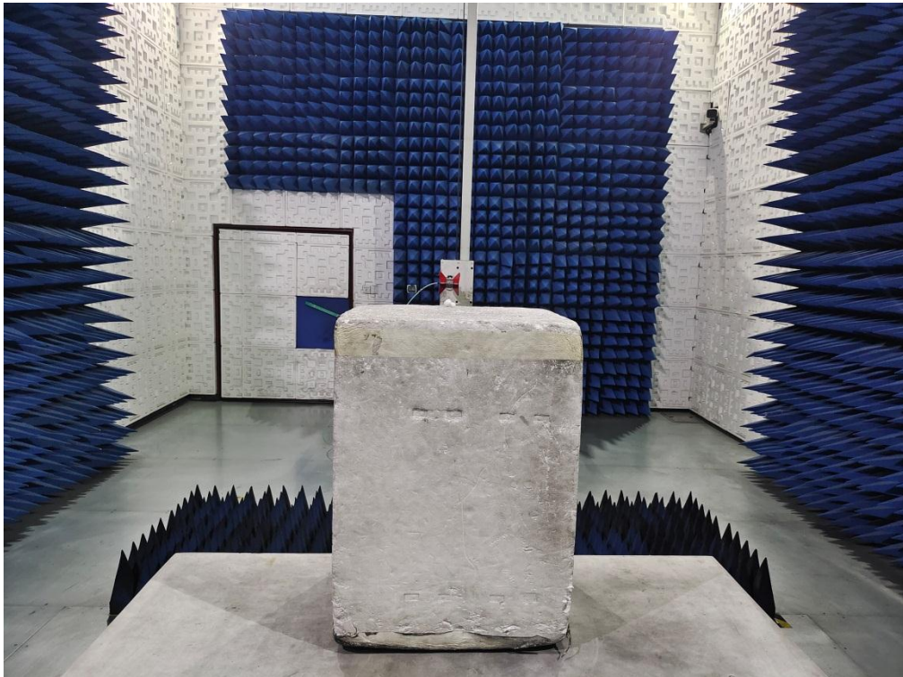
RADIATED EMISSION TEST SETUP ABOVE 1GHz
