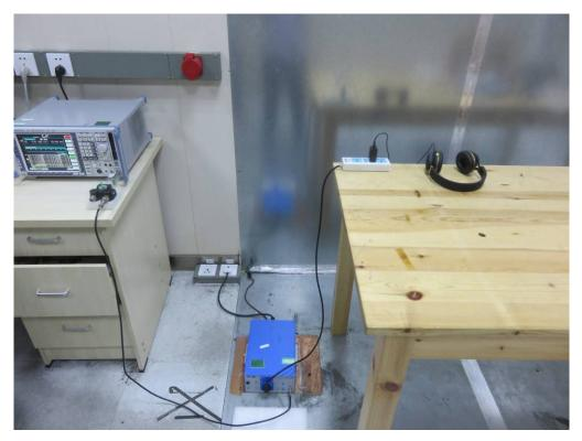
FCC RADIATED EMISSION TEST SETUP
