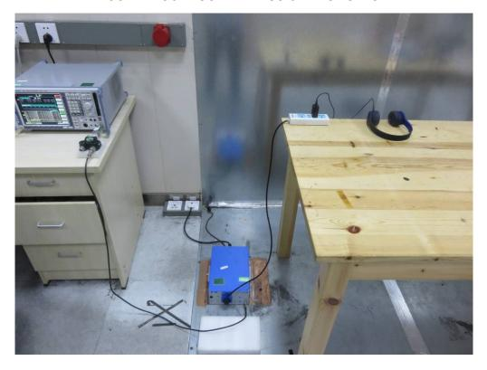
FCC RADIATED EMISSION TEST SETUP
