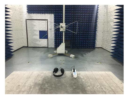
RADIATED EMISSION TEST SETUP ABOVE 1GHZ
