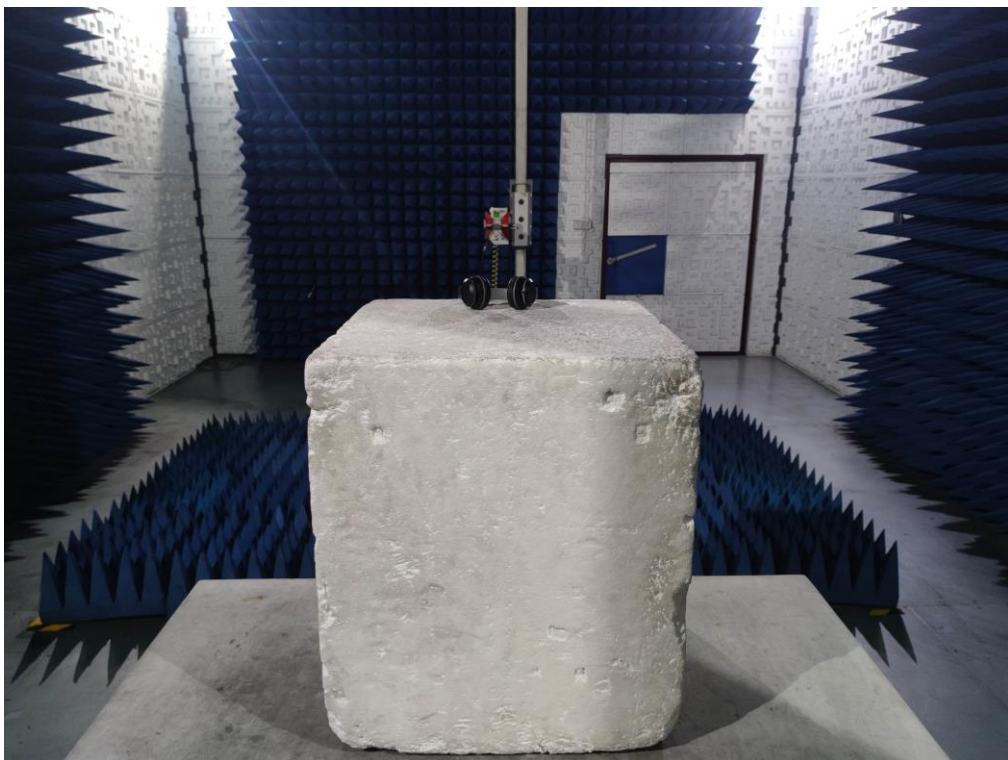
RADIATED EMISSION TEST SETUP ABOVE 1GHz
