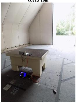
Radiated emissions, Pre-scan, 30 MHz to 1000 MHz
