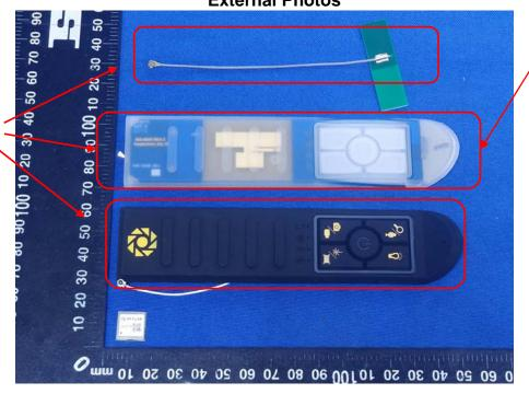
The test antenna which has the wost result
