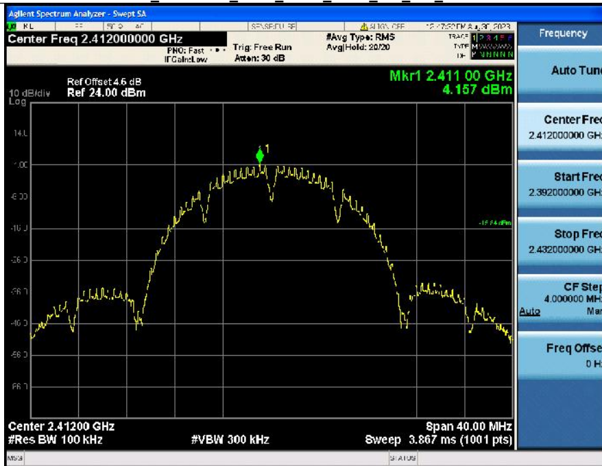
2 Spurious Emission NVNT_ANT1_802_11b_2412
