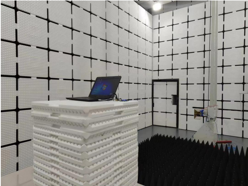
Radiated Emission Test Setup Photo - Above 1GHz
