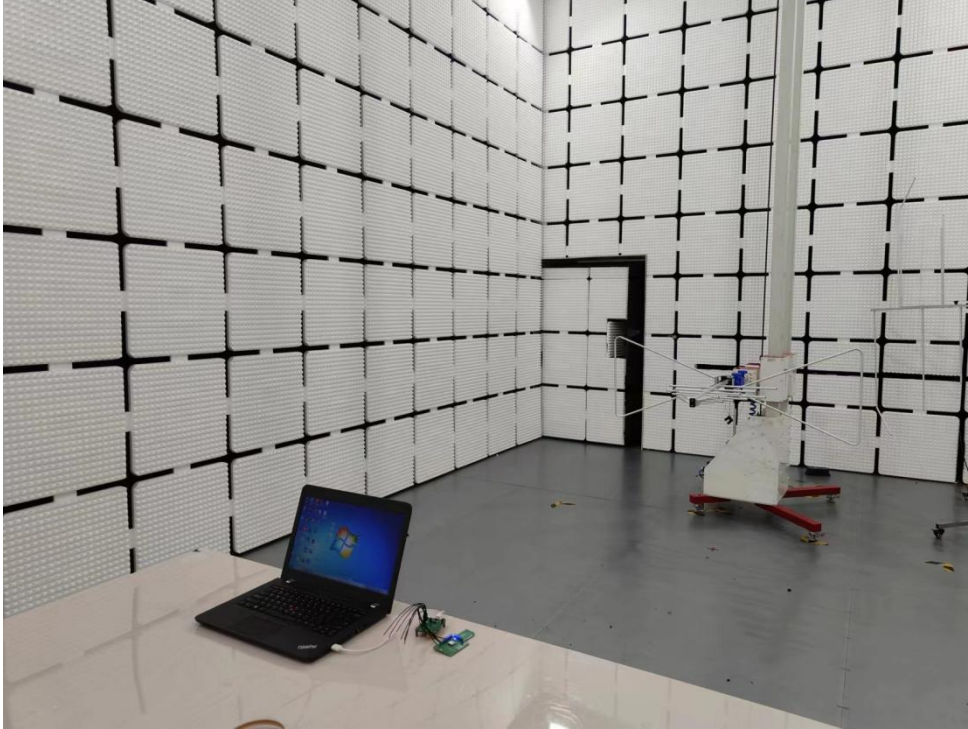
Radiated Emission Test Setup Photo - Below 1GHz
