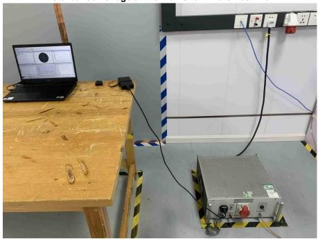
Radiated emission (30 MHz to 1 GHz) Test View
