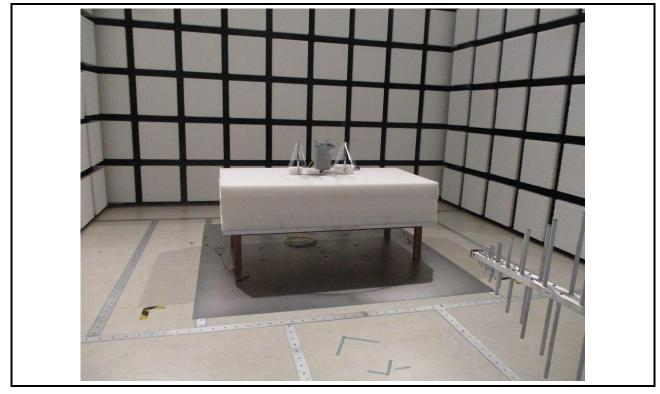
Radiated Emission Below 1GHz Test
