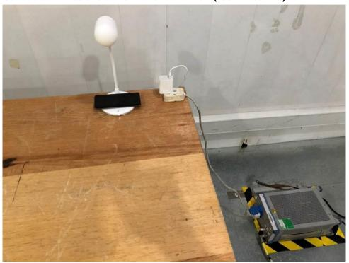
Radiated Emissions (9kHz-30MHz)
