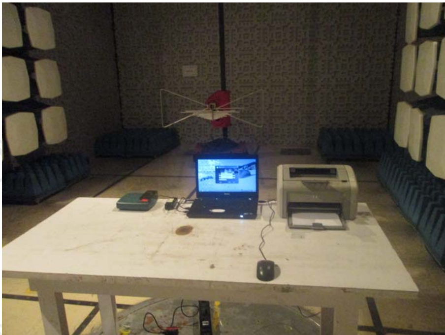
RADIATED EMISSION TEST SETUP-1
