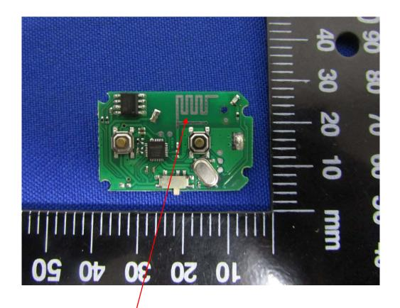
This is a BT antenna, antenna gain is 0dBi.
