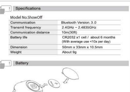
\* Install battery with positive pole facing up.
