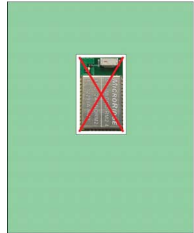
Module placed in center portion of PCB. Not an acceptable design.
