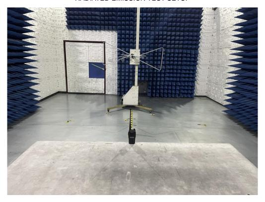
RADIATED EMISSION ABOVE 1G TEST SETUP
