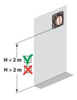
You can also fix the wireless control(s) permanently to the wall with screws.
