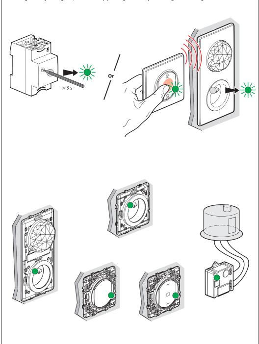
(2) Pair the wireless, batteryless switch to your connected installation.
