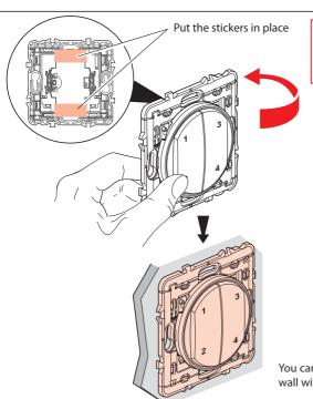
Before fixing the wireless control(s) with the removable stickers provided, test one on a non-visible area of the wall.
