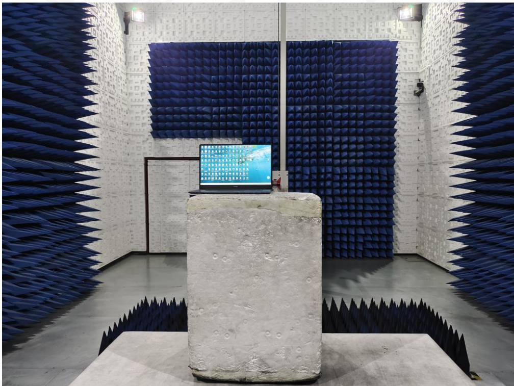
FCC RADIATED EMISSION TEST SETUP ABOVE 1
