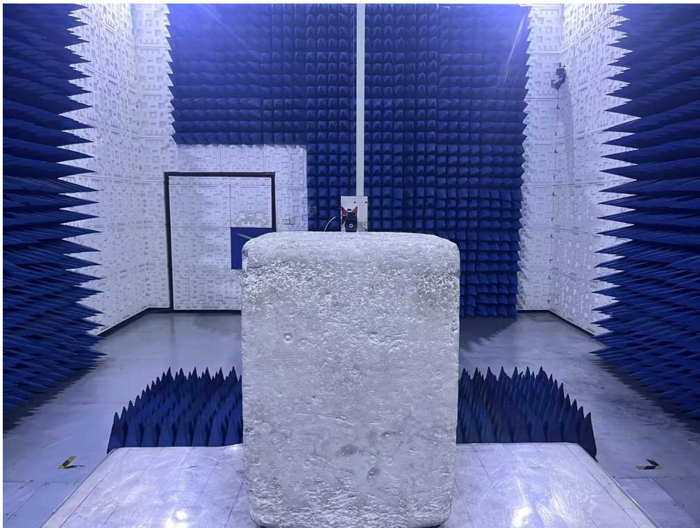
RADIATED EMISSION TEST SETUP ABOVE 1GHz
