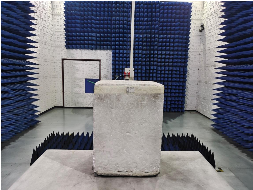
RADIATED EMISSION TEST SETUP ABOVE 1GHZ
