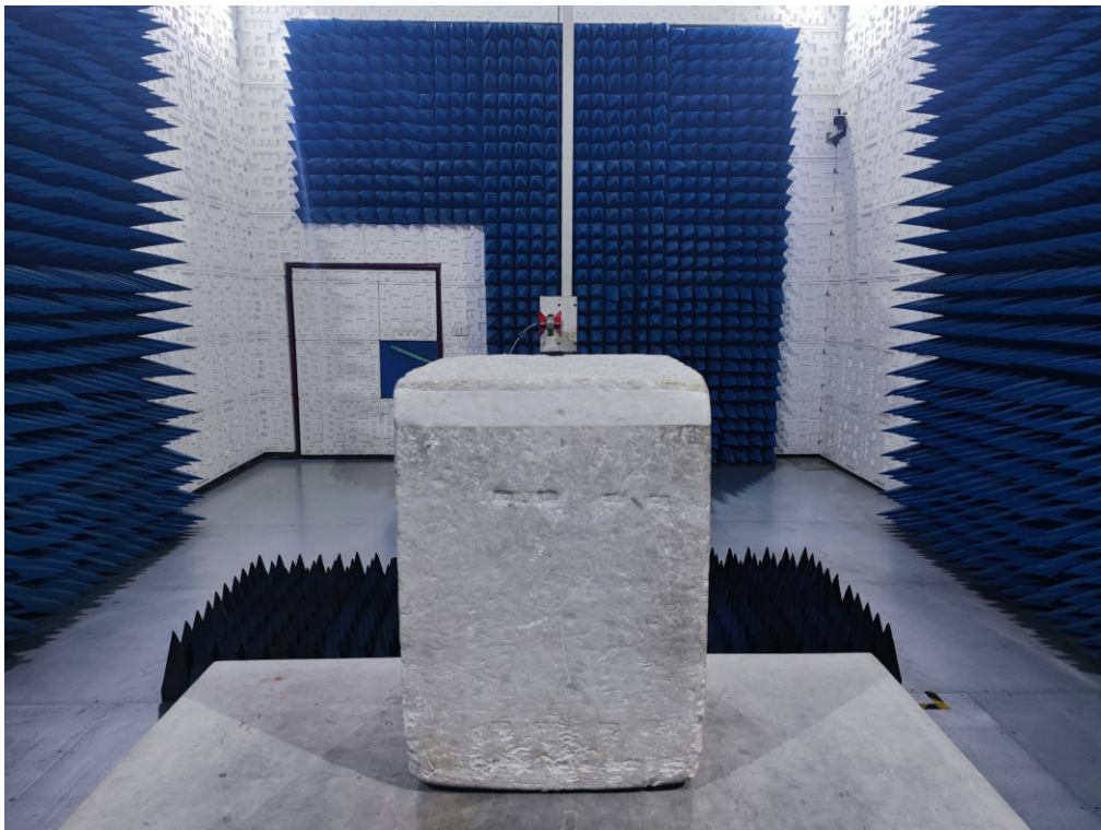
RADIATED EMISSION TEST SETUP ABOVE 1GHZ
